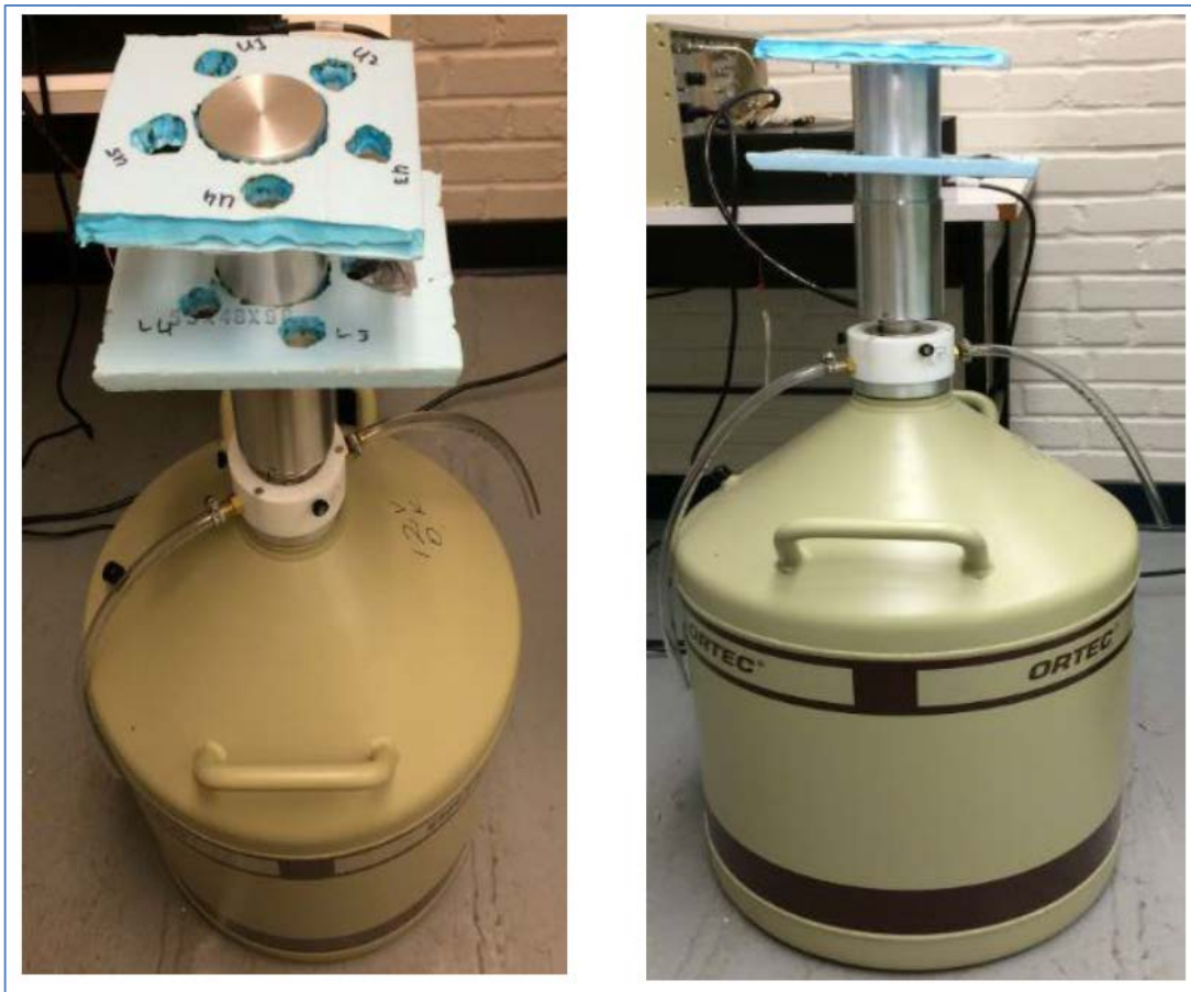
Figure 3. Photograph from Westlake Landfill Tree Core Analysis Report Showing Make-Shift Sample Holder
